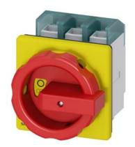
SENTRON, Switch disconnector 3LD, emergency switching-off switch, 3-pole, Iu: 100 A, operating power / at AC-23 A 400 V: 37 kW, front-mounted, rotary operating mechanism, Red / yellow, 4-hole mounting of the handle
