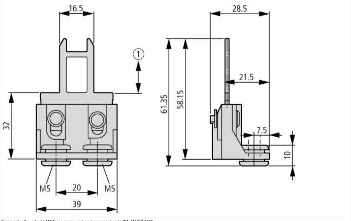
Fixing only allowed with M5 fixing screw and washer according to DIN EN ISO 7093
