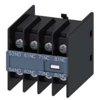
Auxiliary switch on the front, 1 NO + 3 NC Current path 1 NO, 1 NC, 1 NC, 1 NC for contactor relays Size S00 Ring cable lug connection 53/54, 63/64, 73/74, 83/84 Physically coded; only with contactor relays 3RH2140\* and 3RH2440\* can be combined (according to EN 50011)
