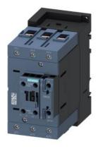
power contactor, AC-3 80 A, 37 kW / 400 V 1 NO + 1 NC, 110 V AC, 50 Hz 3-pole, 3 NO, Size S3 screw terminal
